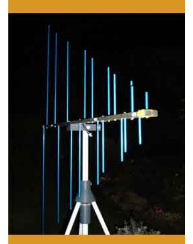
**COMPREHENSIVE** The RF200 is designed to cover the whole range from 30MHz to 1GH in one sweep. No need to change antenna part way through the scan.
