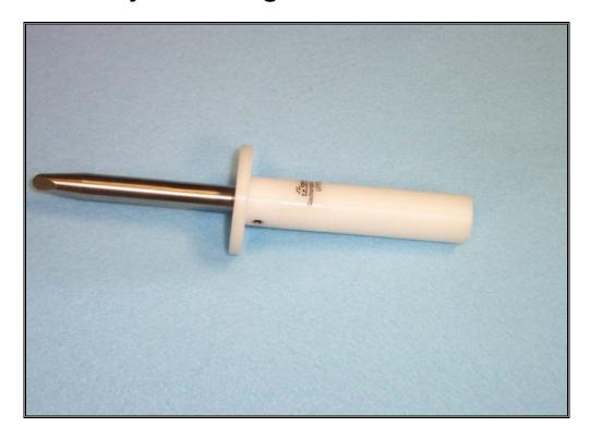
This Unjointed Finger Probe is made for forceful insertion where the flexibility of the Jointed Finger Probe would be difficult. The UFP25 meets IEC 61032 requirements, Figure 7, Test Probe 11. The "finger" portion of the probe is made of stainless steel and the rest of the instrument of Delrin®. The handle is designed with a threaded hole for use with force gauges.
