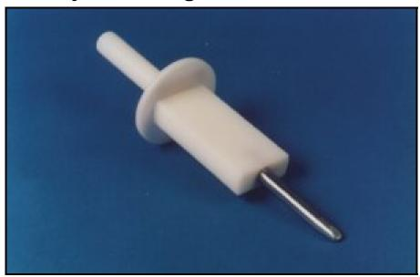
The Unjointed Finger Probe is made for forceful insertion where the flexibility of the Jointed Finger Probe would be a hindrance. The UFP20 meets IEC 60950 and 61010, CSA and UL requirements. This probe is made of stainless steel and the rest of the instrument of Delrin®. The handle is designed with a threaded hole for use with force gauges.
