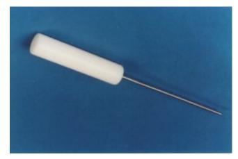
The **3 mm Jewelry Probe** tests to IEC 61010-1, Clause 6.2.3 and others. Material is stainless steel - scribed at 100 mm
