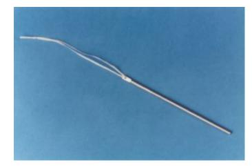
The **4 mm Jewelry Probe** tests to IEC 61010-1, Clause 6.2.2.; IEC 60601, Clause 16(6). String handle is used to hold probe in vertical position for testing. Material is stainless steel - scribed at 100 mm.
