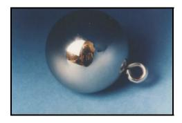
The **Impact Test Ball** is a specially machined ball to test impact resistance according to IEC, CSA and UL Standards. It is made of chrome-plated steel for durability, and is fitted with an eyelet to facilitate testing for pendulum applications. This is called out in IEC 60950, 61032, UL 1989, UL 1418.
