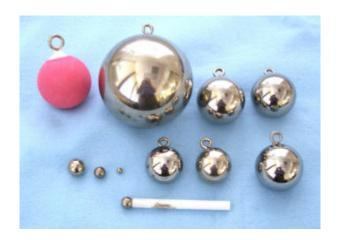
The Impact Test Ball is a specially machined ball to test impact resistance according to IEC, CSA and UL Standards. It is made of chrome-plated-steel for durability, and is fitted with an eyelet to facilitate testing for pendulum applications. Eyelet is threaded to the ball to allow attachment of a handle or force gauge. Weights are closely controlled. Other impact test balls are made without the eye, with a handle and/or made of rubber. See chart below. Contact us for more information.
