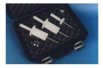
Accessibility probes are used to test the size of openings to ensure that fingers and objects do not have access to hazardous parts in equipment and machinery.
