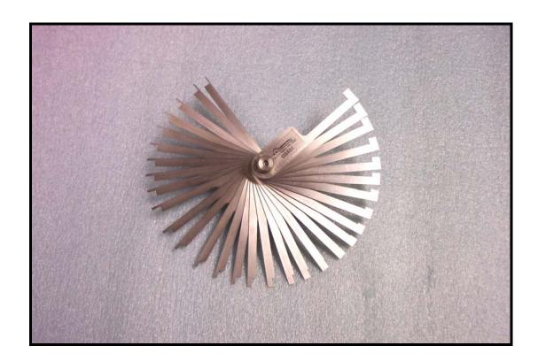
The Gauge Set measures creepage and clearance distances of insulation and spacings of electronic equipment and other products as required by all international standards. There are 31 gauges: 0.6 to 2.0 mm in steps of .1m; and 2.5 to 10.0 mm in steps of .5 mm. Tolerance +0 /-0.02 mm. Extra small gauges have been added to measure modern printed wiring distances. Made of stainless steel.
