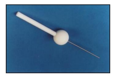
The **Test Rod Probe** tests to IEC 60529 and 61032, Figure 3, for protection against access to hazardous parts with a tool. The rod is made of stainless steel and the stop face and handle are made of Delrin®. Probe is 100 mm. long and 2.5 mm in diameter.
