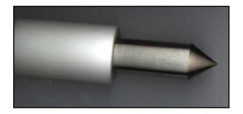
The **Test Thorn Probe** is used for testing appliances according to IEC, CSA and UL Standards. This probe is made of stainless steel with a Delrin® handle. It is used to verify protection from hazardous hot or glowing parts.
