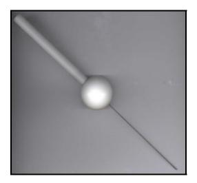
The Test Wire Probe, 1.0 mm. in diameter, is used to test to IEC60529 for protection against access to hazardous parts with a wire. This probe is made of stainless steel with a Delrin® handle.
